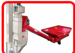
Reception through swing away hopper, with option of precleaning
